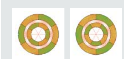
Fig. 2 Radial-flux type PMC when aligned Fig. 3 Torque produced due to Push-Pull
